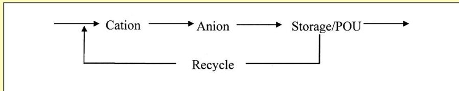
Figure 2 – A fraction of the DI water is recirculated to the front of the deionizer to maintain the water's purity.
